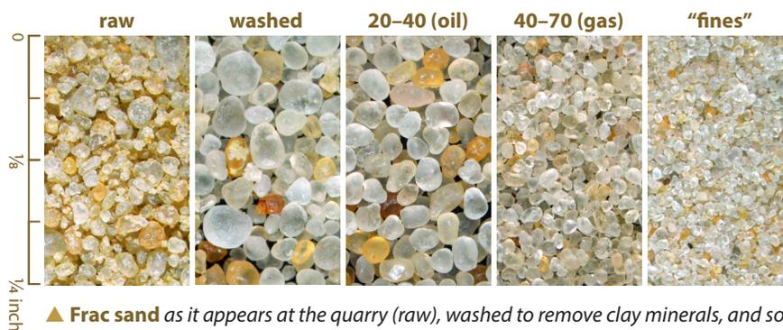
▲ **Frac sand** as it appears at the quarry (raw), washed to remove clay minerals, and sorted by size for various uses (number ranges identify openings per inch in the sorting sieves). Sand that is too small for use in hydraulic fracturing (“fines”) may be used as fill for mine reclamation, as cow bedding, or for other purposes.
